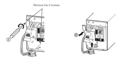
4. Hold the pullout label at the bottom of the battery pack and remove the battery pack.
